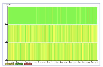
The diagrams (made on an dual core MacBook laptop), shows that in the first case parallelising is efficient and master successfully distributes load to workers, while in the second case a single computation is just too short, so most of the time is spent on communication. To parallelize the Euler's function example efficiently, tasks must rather be grouped in chunks, which should be enough large to reduce the communication overload, but enough small to ensure that tasks are evenly distributed.
